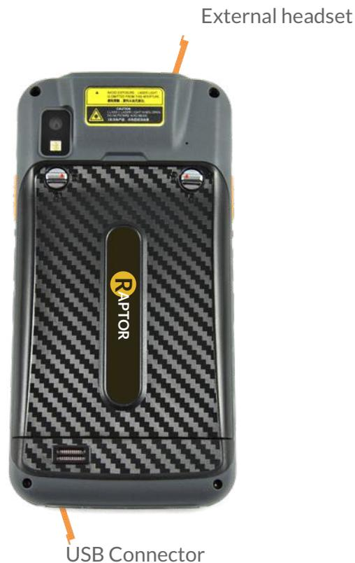
All connectors have rubber covers which are required to maintain the IP rating of the device.
