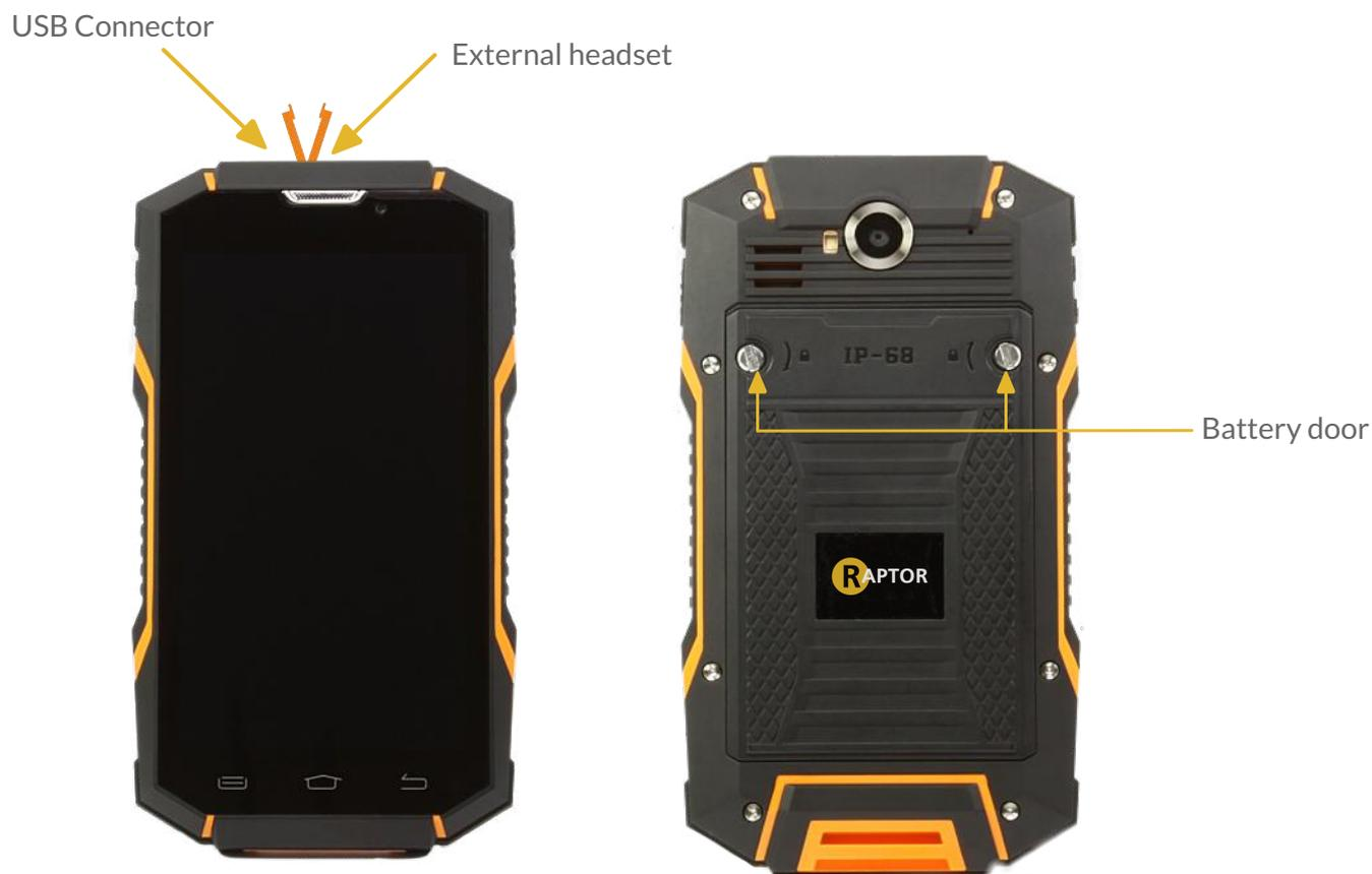
**Connector rubber covers** - Must be kept securely fitted at all times to ensure maximum IP rating of the device. When using connectors, make sure to only use supplied accessories and be careful to not allow water or dust to enter the device.
