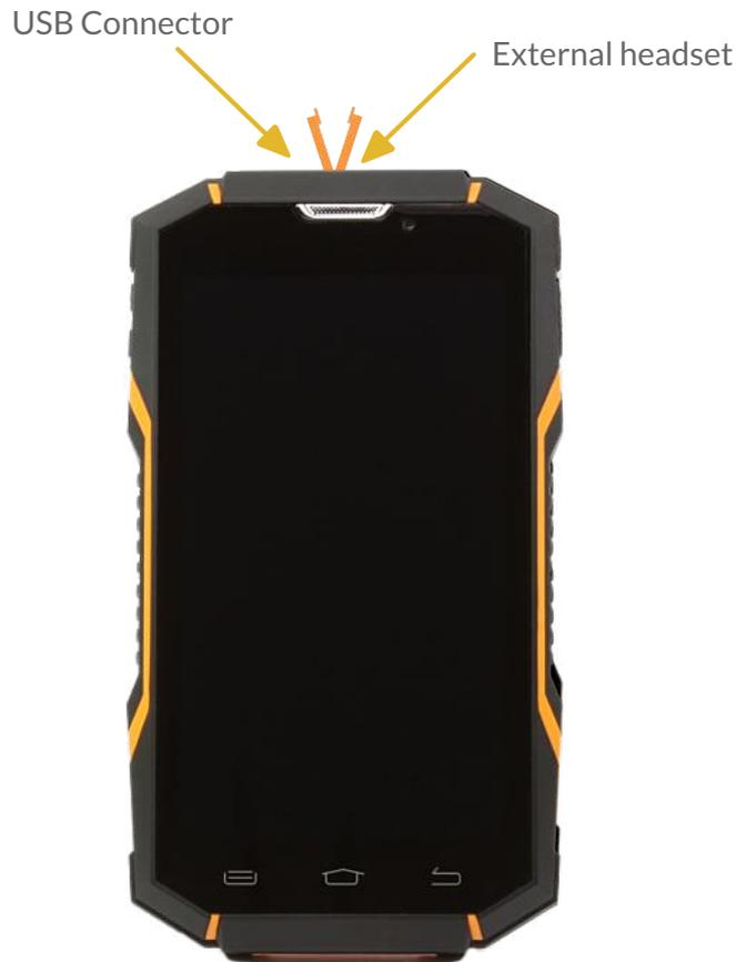
All connectors have rubber covers which are required to maintain the IP rating of the device.
